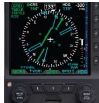
Figure 2-47 BRG#1 Set to VOR1 on 117.9; BRG#2 Set to GPS2, SWR
