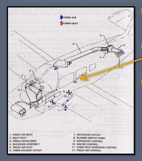
Airflow is regulated between front and rear seats by levers
