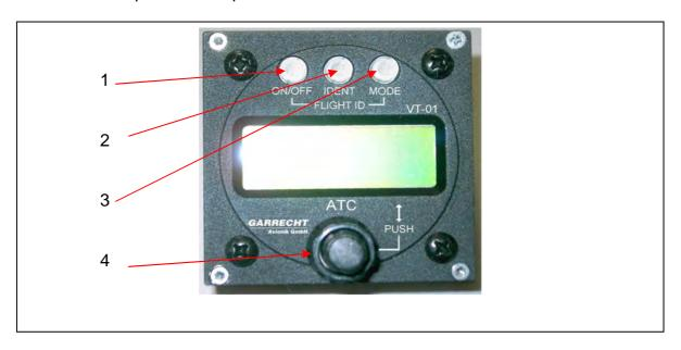
The system will be operated using the following devices:
