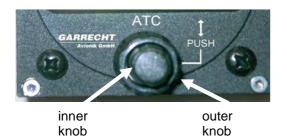
Select the position to be modified by rotating the outer knob. The selected position will be indicated by a blinking cursor
