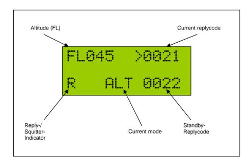
The current pressure altitude (related to 1013,25 hPa) will be shown as Flightlevel (FL) in the upper left corner of the LCD screen.
