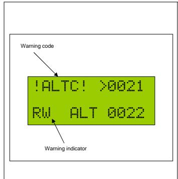
In case of warning, the system shows a union the LCD screen. Additionally, a frequently repeated audible signal occurs. Both can be terminated by pressing the on/off key shortly.
