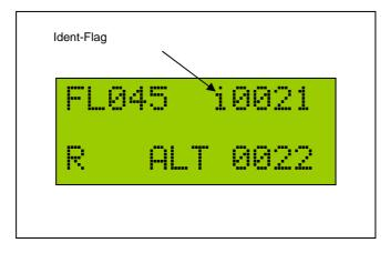
Pressing the ident key invokes the ident mode for 18 sec. Ident activity is shown by a **i** in the middle of the upper line on the LCD screen, which starts blinking after 4 sec. as long as ident is acitve.
