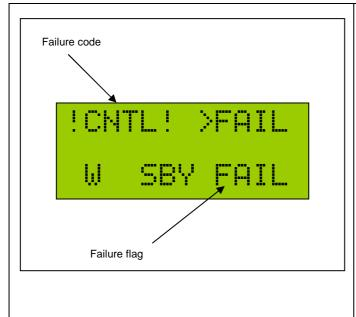
In case of failure, the system shows a ... on the LCD screen. Additionally, a frequently repeated audible signal occurs. Both can be terminated by pressing the on/off key shortly.
